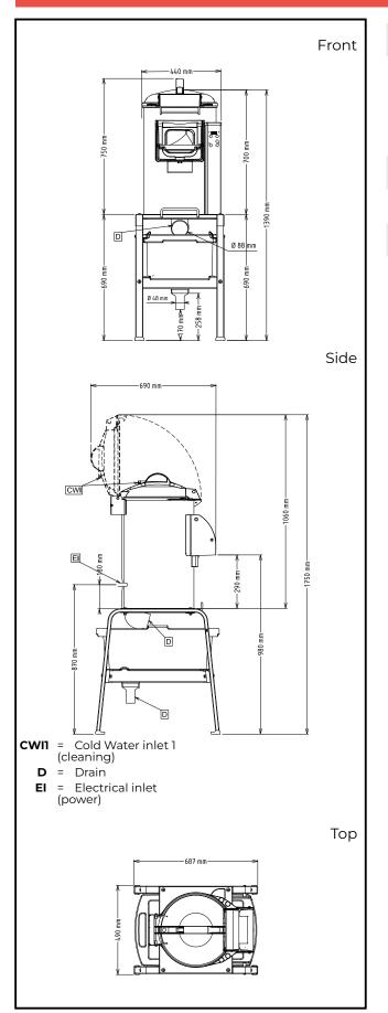
Electric Supply voltage: 603511 (DT15E1) 220-240 V/1N ph/50/60 Hz 200-240/380-440 V/3 603512 (DT15E324) ph/50/60 Hz Electrical power, max: 0.37 kW 0.37 kW **Total Watts:** Capacity: Performance (up to): 240 kg/Cycle Capacity: 15 litres Key Information: External dimensions, Width: 440 mm External dimensions, 690 mm Depth: External dimensions,
